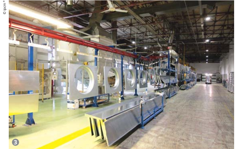
Figure 3: After machining, the galvanised sheet metal fairings are sent to the pre-treatment tunnel.
